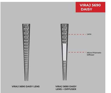
**VIRAJ 5690 DAISY** Linear Luminaire in a sleek design with a slim Extruded aluminium housing and with premium powder coating finish.
